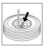
Tilt the retainer and slip it through the wheel opening when the spare tire has been completely lowered.
